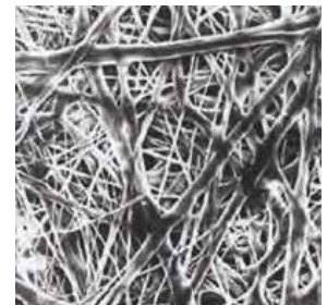
Tough, continuous fibers create a tortuous path for superior barrier properties.
